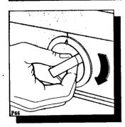
Press and turn the programme dial clockwise until letter A on the dial coincides with the red marker line.
